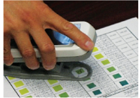
Figure 2—Ihara color densitometer.
